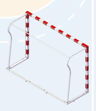
The stabilizer system is composed on the one hand of lateral supports (arches) rigidized with a tube at the top and, on the other hand, of the rectangular base with rods to hold the net, and 4 anti-overturn sheets, all of them, joined to the frame trough screws.
